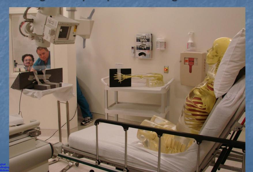
We did this experiment with and without grids, at 115 and 85 kV, and at 3 different angles.
